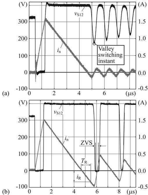
Fig. 4. Measurement results of a boost cell (a) without and (b) with an extended reverse conduction time  $T_R$  [cf., Fig. 3(b) and (c)]. In order to minimize the switching losses, (a) valley switching can be applied, whereas the extension of  $T_R$  allows for (b) ZVS over the complete mains period. (Parameters:  $v_n = 328$  V,  $V_{out} = 400$  V, and  $T_{on} = 750$  ns).
