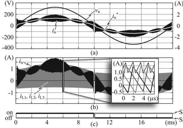
Fig. 9. Simulation results for a 200 W three-cell PFC rectifier system [cf., Fig. 2(b)]. (a) Mains voltage  $v_n$ , input current  $i_n$ , and first-order low-pass filtered input current  $i_n^*$  ( $f_c = 16$  kHz). (b) Inductor currents including a magnified view which shows the smoothing effect of the superposition on the input current  $i_n$ . (c) Gate signals of the low frequency switching bridge-leg.
