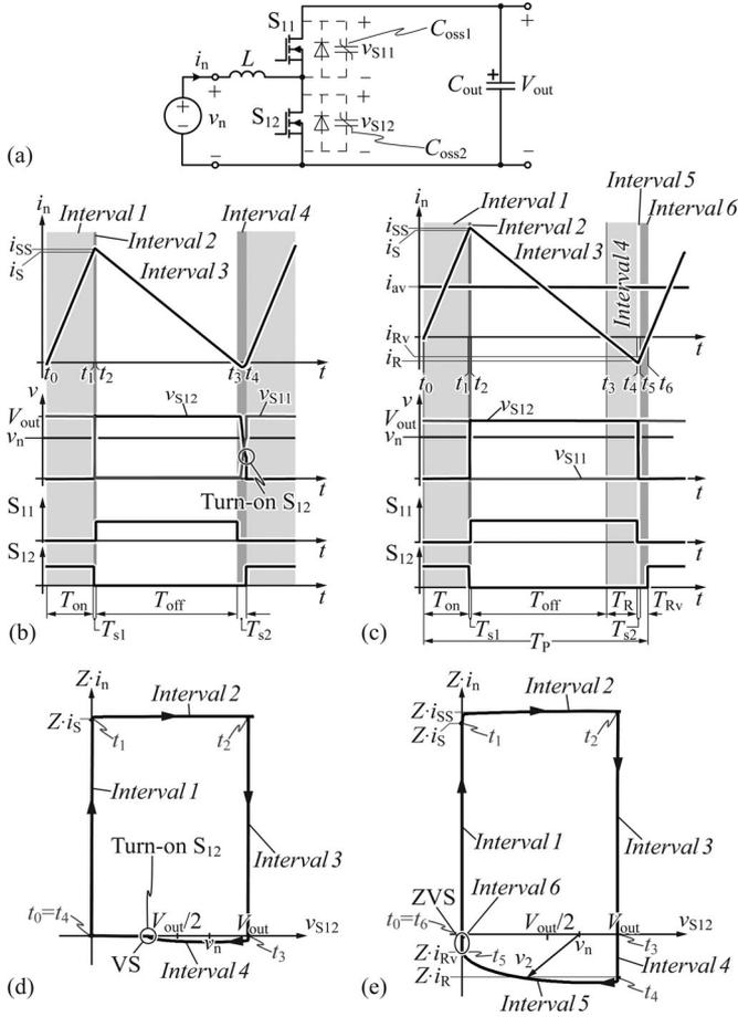
Fig. 3. (a) Single-cell configuration during the positive half-line cycle. (b) Current and voltage waveforms for valley switching. (c) Current and voltage waveforms for the proposed ZVS strategy. A detailed view of the switching transition in intervals 4 and 5 is given in Fig. 6. (d)  $V$ - $Zi$  plot for valley switching. (e)  $V$ - $Zi$  plot employing ZVS.
