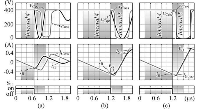
Fig. 6. Comparison between different capacitor models used to describe the nonlinear output capacitances of the MOSFETs. In simulations, each model is compared to the nonlinear capacitance given in the datasheet of the switch. (a) Energy equivalent linear capacitance, (b) charge equivalent linear capacitance, and (c) proposed charge model (13) of the capacitance. For each model, the corresponding current value  $i_R$  is calculated in order to achieve ZVS.
