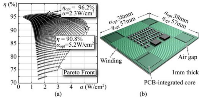
Fig. 14. (a)  $\alpha$ - $\eta$ -Pareto front of a PCB-integrated boost inductor, which allows for an ultraflat realization of the converter system. A detailed description of the design procedure is given in [37]. (b) Three-dimensional sketch of a PCB-integrated boost inductor. The dimensions are given with respect to the two optima indicated in (a). Due to the large winding window, several components could be placed within the boost inductor in order to increase the power density  $\alpha$ .
