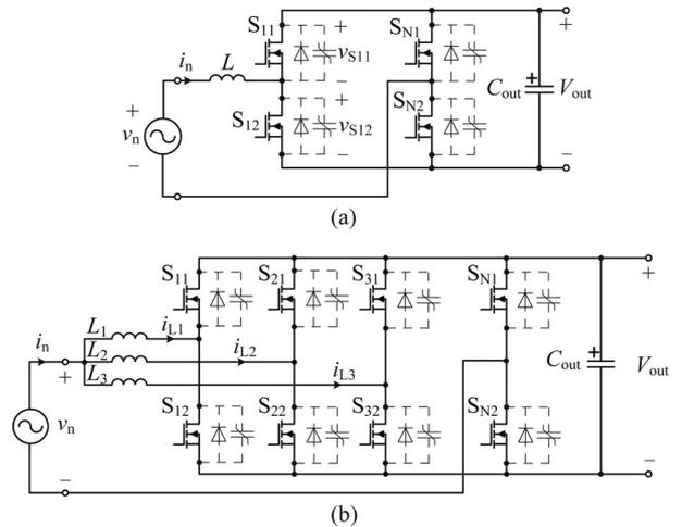
Fig. 2. (a) Single-cell and (b) three-cell configuration of a TCM PFC rectifier system employing ZVS over the entire mains period.
