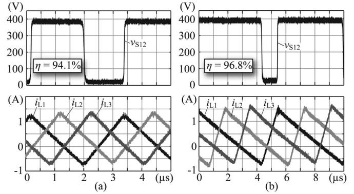
Fig. 12. Measurement results of converter system operating in dc–dc mode. The figure shows that each bridge-leg operates in ZVS mode and that the interleaving of the inductor currents is properly achieved with the presented interleaving control method. (a)  $v_n = 230$  V,  $V_{\text{out}} = 400$  V, and  $P_{\text{out}} = 200$  W. (b)  $v_n = 325$  V,  $V_{\text{out}} = 400$  V, and  $P_{\text{out}} = 400$  W.
