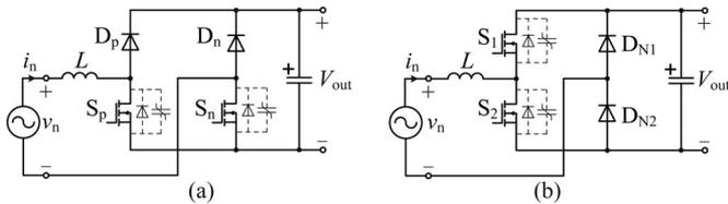
Fig. 1. (a) Bridgeless PFC rectifier with parasitic output capacitances of the MOSFETs.  $D_p$  and  $S_p$  shape  $i_n$  for  $v_n > 0$  whereas  $D_n$  and  $S_n$  shape  $i_n$  for  $v_n < 0$  [16]. (b) Totem-pole bridgeless PFC boost rectifier [16].
