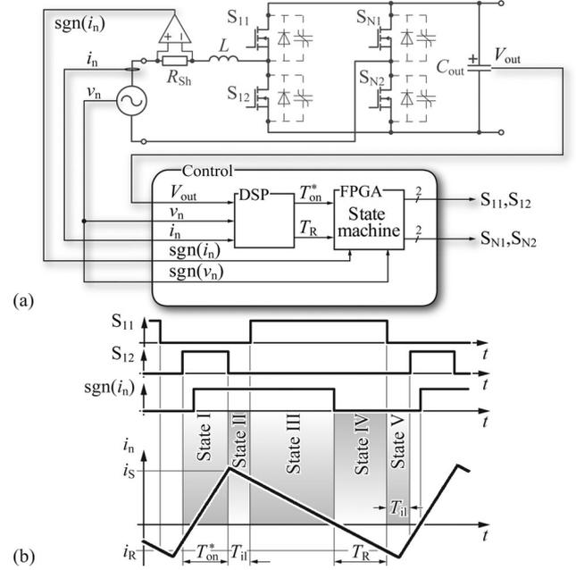
Fig. 8. (a) Schematic and simplified control structure of a single-cell TCM PFC rectifier which shows all required measurements. (b) State machine goes through each stage. It requires  $T_{on}^*$  and  $T_R$  which are determined in the DSP and the zero-crossing signal of the inductor current. A constant interlock delay  $T_{il}$  is considered.
