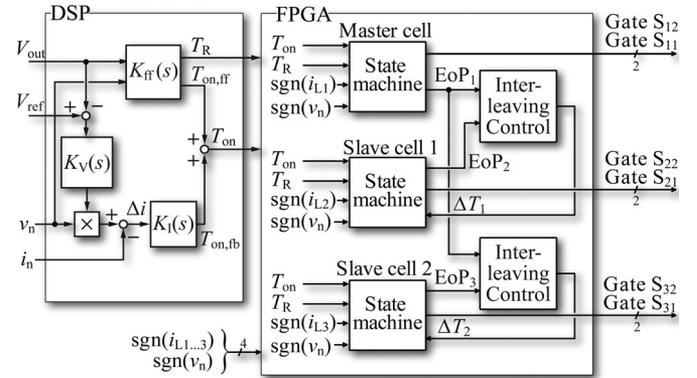
Fig. 11. Schematic of the control structure of the converter system which is subdivided into the state machine of each HF bridge-leg and the interleaving control of the inductor currents which are implemented in an FPGA and a superimposed input current and output voltage control realized in a DSP.
