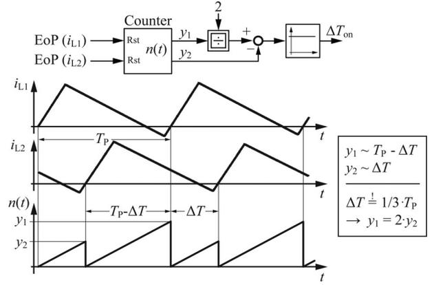
Fig. 10. Evaluation of the control signal for the interleaving control which is based on the EoP signals of each inductor current  $i_{L1} - i_{L3}$ . A counter is reset at EoP of each current and the values are then compared to each other.
