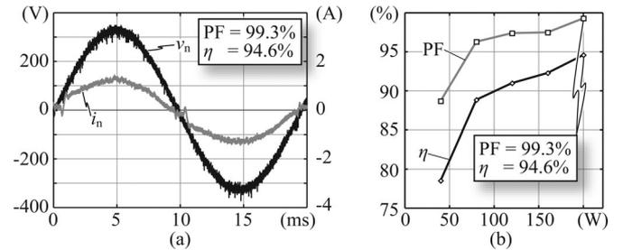
Fig. 13. (a) Input voltage  $v_n$  and input current  $i_n$  of the TCM PFC rectifier ( $V_n = 230$  V,  $V_{\text{out}} = 400$  V,  $P_{\text{out}} = 200$  W). (b) Efficiency  $\eta$  and power factor PF as a function of the output power  $P_{\text{out}}$ .
