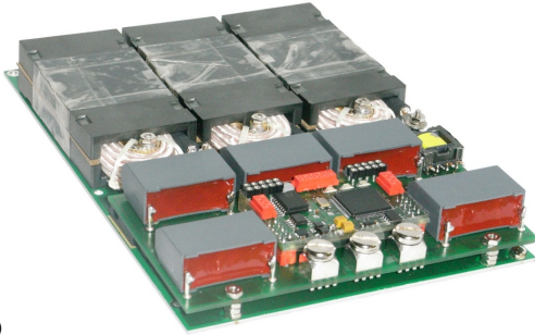
Fig. 10: a) 6 kW dc-dc 3-interleaved buck converter hardware prototype and b) main waveforms ( i_{L,DSP} : 30 A/div, i_{L1} : 5 A/div, u_G : 10 A/div).
