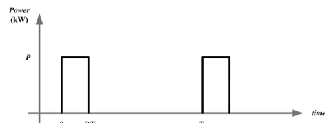
Figure 1 – A generalized high peak load low duty cycle power profile, with peak power P and period T much greater than on time DT .
