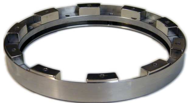
Figure 4: Open rotor of the prototype system. Shown is the ferromagnetic ring with the rotor magnets on top, enclosed by the rotor shell made of stainless steel.
