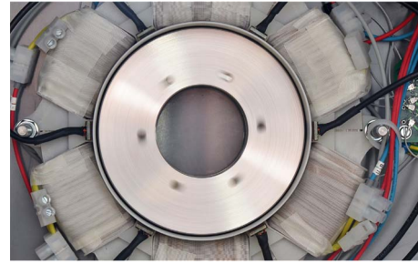
Fig. 16. Spinning rotor seen from above. To each side, the rotor has a free air gap of 1 mm. Rotational speeds of up to 20 000 r/min are tested.
