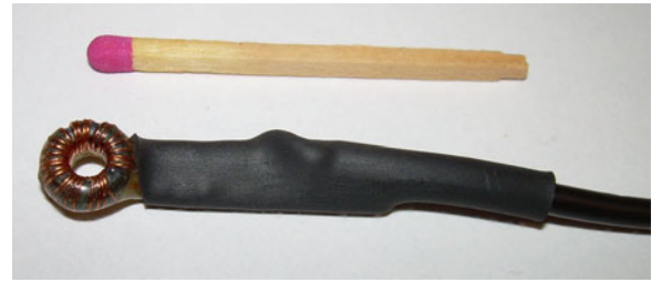
Fig. 11. Constructed ac current transformer with a sensitivity of 100 mV/A to measure the drain-source current I_{DS} of the MOSFET.
