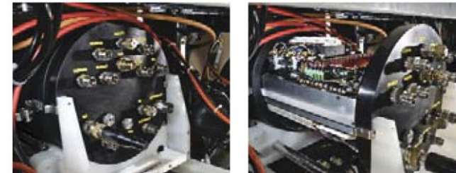
Electronics Compartment of Seaeye Jaguar
