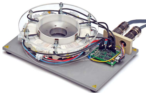
Fig. 9. Picture of prototype A with six coils and diametrically magnetized rotor. The annular rotor has an outer diameter of 102 mm and a total height of 18 mm.
