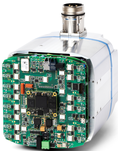
Figure 12. Photograph of the complete motor-integrated, MPPB-operated, single-phase-supplied, variable-speed-drive system of Figure 1.
