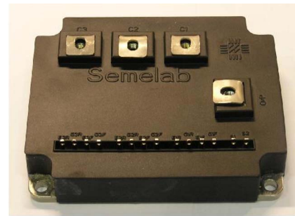
Fig. 8. Semelab 300-A 600-V 3 × bidirectional switch module developed for the EDAAS project.
