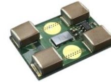
Source: R. Pilawa Integrated Dual-Sided Half-Bridge Flying Capacitor Converter Switching Cell
