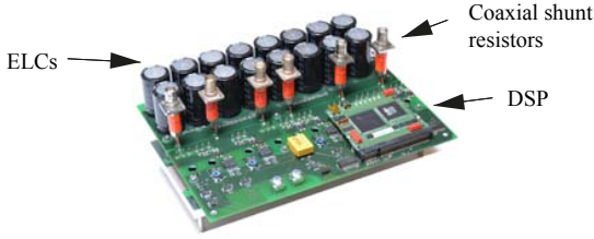
Fig. 9. The switching loss measurement setup.
