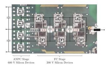
**Fig. 8.** Realization of the hardware layout of a three-phase 7L-HANPC inverter bridge leg, where the FCs (film-type) are placed underneath the PCB, and ceramic capacitors are placed on top to improve the switching behavior of the MOSFETs. The commutation loop introduced by the connection the FC stage to the HANPC stage  $L_{c3}$  is the most critical.
