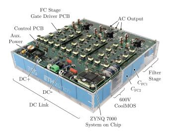
**Fig. 7.** Hardware prototype of the 12.5 kW three-phase 7L-HANPC inverter, measuring  $256 \text{ mm} \times 269 \text{ mm} \times 53 \text{ mm}$  (10.1 in  $\times$  10.6 in  $\times$  2.1 in). The final volumetric power density is  $3.4 \text{ kW/dm}^3$  (55.9 W/in<sup>3</sup>), and the gravimetric power density is 3.2 kW/kg.
