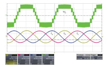
**Fig. 9.** Measurements of the seven-level output voltage of a bridge leg of the 7L-HANPC inverter shown in **Fig. 7** (200 V/div, referenced to the DC-link midpoint voltage, 5 ms/div) and the three phase mains currents (20 A/div) during operation at 10 kW.
