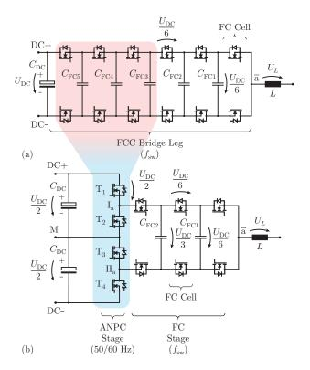
**Fig. 2.** Topology of a 7L-FCC bridge leg, which is purely composed of low-voltage semiconductors operated at switching frequency (**a**) and the 7L-HANPC bridge leg structure, which is a hybrid approach composed of an ANPC stage with semiconductors switching at 50/60 Hz, and a FC stage, with semiconductors operating at switching frequency (**b**); both arrangements are shown for phase a of the three-phase (phases a, b, c) inverter topology.
