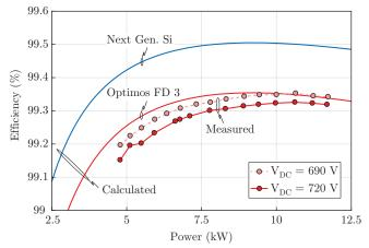
**Fig. 10.** Measured efficiency of the hardware demonstrator (cf. **Fig. 7**) reaching peak values of 99.35% for  $U_{\rm DC}$  = 690 V and 99.32% for  $U_{\rm DC}$  = 720 V, and the calculated efficiency for the prototype with the current semiconductor configuration at  $V_{\rm DC}$  =720 V and with the configuration using *next generation* silicon switches from *Infineon* (solid lines), which will reach a peak efficiency of 99.5%.
