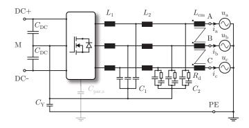
**Fig. 5.** EMI filter structure of the final prototype, with two L-C filter stages attenuating DM and CM components of the output voltages of the inverter bridge legs (with reference to the DC voltage midpoint) and a CM choke placed before the grid connection.
