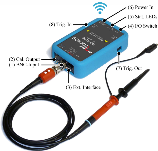
Fig. 7: Prototype of the wireless oscilloscope with physical dimensions of 141 mm × 81 mm × 32 mm. Front side: (1) BNC connector for the input signal, (2) calibration signal output and (3) interface for external sensors; back side: (4) I/O power switch, (5) status and charge indication LEDs and (6) connector for the battery charger; left/right side: (7) optical trigger out- and (8) inputs.
