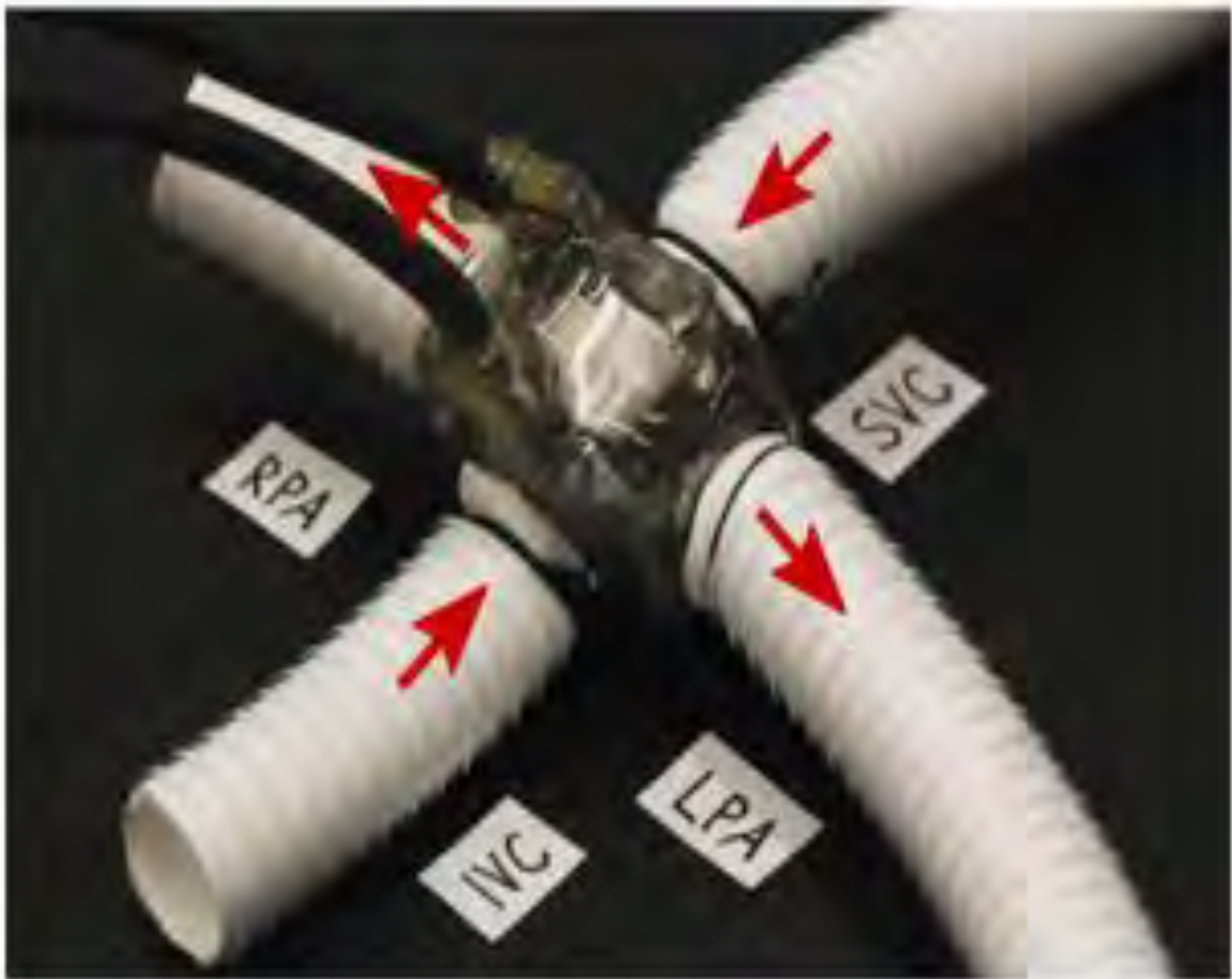
Physical prototype of the CPAD designed to assist the Fontan circulation by pumping blood via DOME-TEX ® vascular grafts from the caval veins (IVC: inferior vena cava; SVC: superior vena cava) into the pulmonary arteries (LPA: left pulmonary artery; RPA: right pulmonary artery). The red arrows indicate the direction of blood flow. The CPAD features a total volume of 1.7 liter 3 with the distal ends of the cannula in- and outlets being spaced by 34 mm and 40 mm, respectively.
