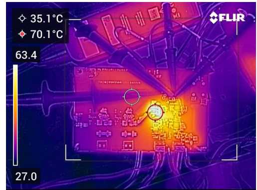
Fig. 8: Measurement results of DCX stage: (a) Waveforms of the DCX operating at 300 V dc input, 52 V dc output, and 240 W. (b) Thermal image at the same operating point focusing on the semi-conductors.
