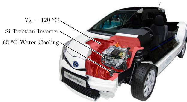
Fig. 1. Toyota Hybrid Synergy Drive in a Yaris Hybrid of the model year 2012: Industrial example of a traction inverter with Si IGBTs which is placed under the engine hood with ambient temperatures up to 120 °C and hence requires a low temperature water cooling circuit. (Photograph taken at the world premiere of the Toyota Yaris Hybrid at the 82nd Geneva International Motor Show in March 2012.)
