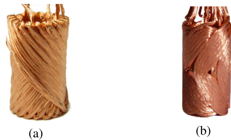
Fig. 1. Skewed winding (a) and rhombic winding (b)
