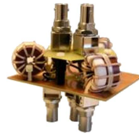
Fig. 11. Three-phase CM/DM separator prototype photograph. Overall dimensions: 7.0 \times 7.0 \times 8.2 cm ( 2.8 \times 2.8 \times 3.2 in).
