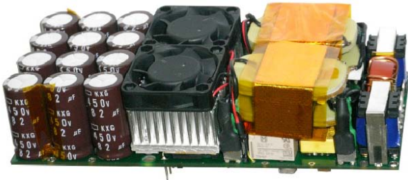
Fig. 22: Laboratory prototype of the ultra-compact 3.2kW dual-boost PFC rectifier according to Fig. 9b) composed of two interleaved 1.6kW units; overall dimensions: 175x80x42mm; output power density: 5.5kW/l.
