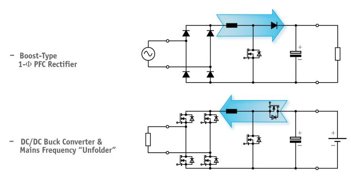
Low-Frequency "Folder/ Unfolder" vs. PWM Operation of Output Stage
