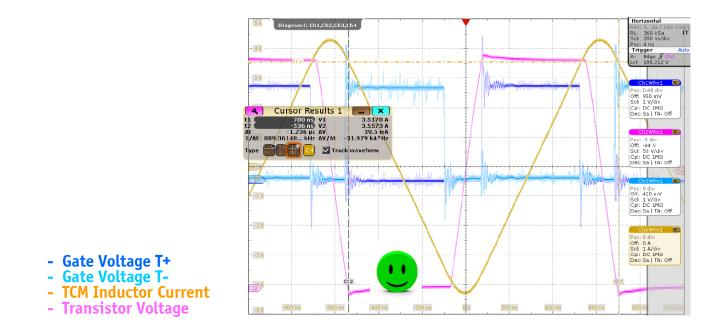
• Triangular Current Mode (TCM) Operation at No Load  $\rightarrow$  ZVS and No Free Ringing of  $u_{T+}$ ,  $u_{T-}$  or  $i_{L}$
