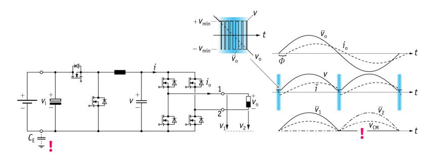
PWM Operation of Mains Frequency Inverter @ U < U<sub>min</sub>
