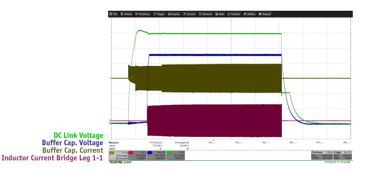
Start-up and Shut-Down (No Load Operation)
