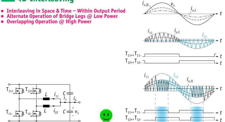
• Opt. Trade-Off of Conduction vs. Switching Losses / Opt. Balancing of Thermal Stress
