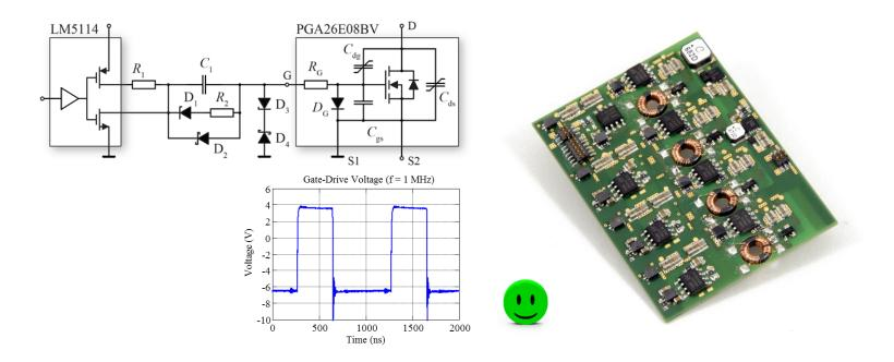
Total Prop. Delay < 30ns incl. Signal Isolator, Gate Drive, and Switch Turn-On Delay
