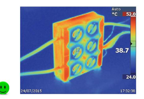
**Two-Side Cooling**  $\rightarrow$  Heatsink Temperature = 52°C @ 80W (8W Natural Convection)
