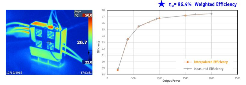
■ Heating of System Lower than Specified Limit (*T*<sub>C,max</sub>= 60°C @ *T*<sub>amb</sub>= 30°C)
