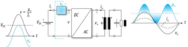
Parallel Approach for Limiting Voltage Stress on Converter Stage Semiconductors
