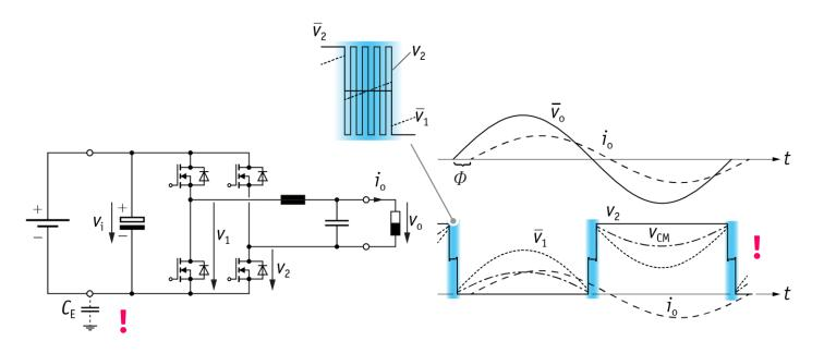
PWM Operation of Mains Freq. Bridge Leg @ |u| < u<sub>0,min</sub>
