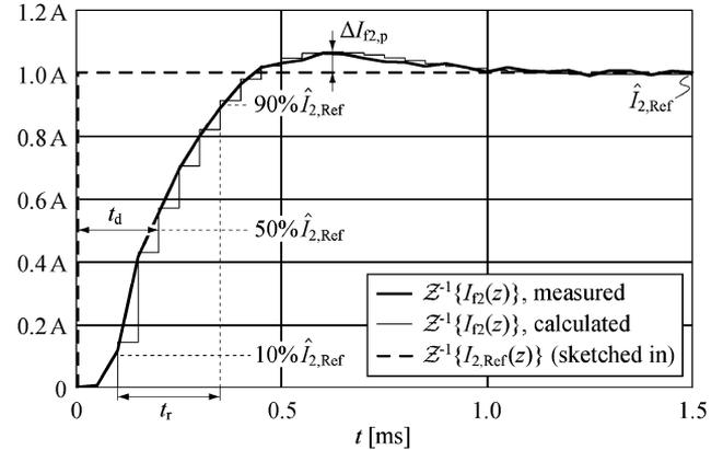
Fig. 15. Measured and calculated unity step response of the closed current control loop; a rise time  $t_r$  of approximately 250  $\mu\text{s}$  and a delay time  $t_d$  of approximately 200  $\mu\text{s}$  are achieved.
