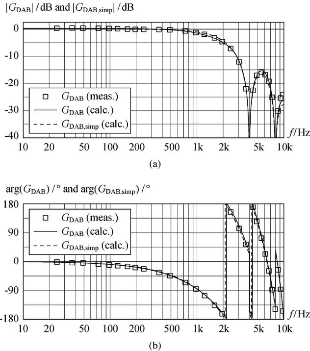
Fig. 14. Frequency response of the accurate transfer function  $G_{DAB}$  (solid lines) and the simplified transfer function  $G_{DAB,simp}$  (dashed lines). (a) Gain and (b) phase diagrams; the boxes mark measured values.
