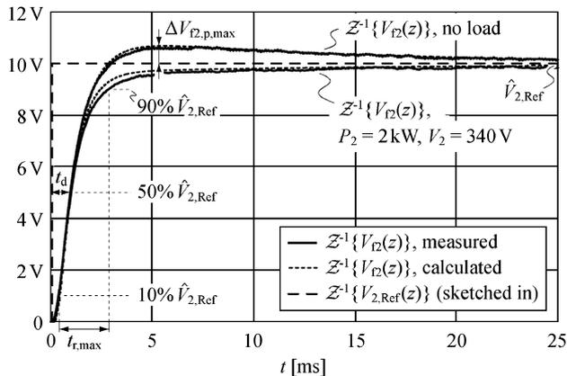
Fig. 16. Step response of the closed voltage control loop for no-load operation and for 2 kW output power at 340 V output voltage; the input voltage is 12 V and the output voltage step amplitude is 10 V.
