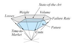
Fig. 1 State-of-the-art and future performance improvement of power electronic systems.
