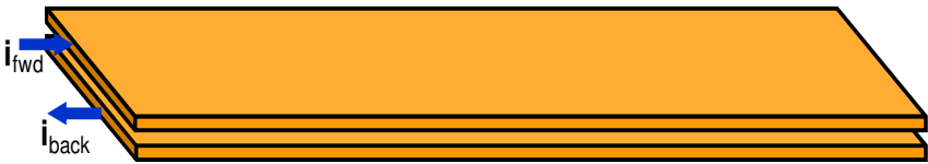
Fig. 1. Principle of bus bar design. Example value: 30mm width, 100mm length and 0.5mm distance will result in an inductance of 2.1nH
