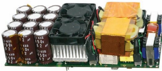
Fig. 14: Prototype of the ultra-compact 3.2kW bridgeless PFC rectifier composed of two interleaved 1.6kW units; overall dimensions: 175mm \times 80mm \times 42mm; output power density: 5.6kW/dm 3 .
