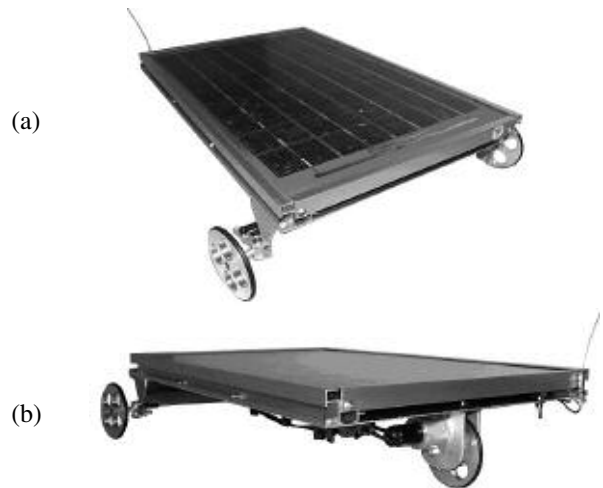
Fig. 3: Model solar car. (a) Front and (b) rear view (dimensions: 41 cm x 35 cm x 10 cm, weight: 2.5 kg)
