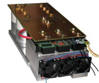
Figure 16. Solid state modulator with 4kA/1kV per switch used for measurements.
