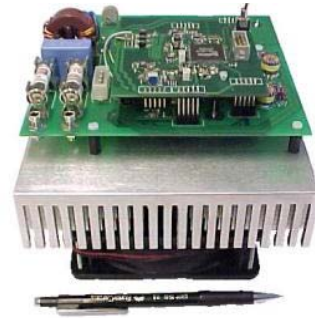
Fig. 8. Prototype of a 5kW/500kHz series-parallel resonant converter with ZCS in one and ZVS in the other leg.
