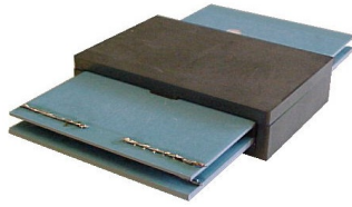
Fig. 10 Prototype of LP z-compressed transformer with PLP
