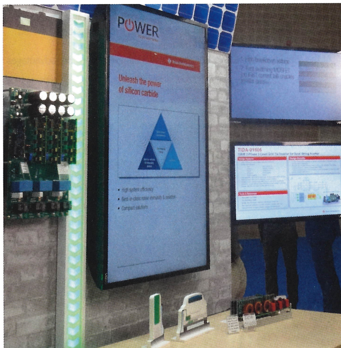
TI's 10 kW, SiC-based grid tie inverter reference design for a transformer-less solar string inverter with 99 % peak efficiency
