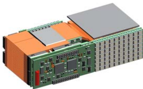
Figure 4. 10kW/liter, 5kW DC/DC converter, 3D CAD drawing
