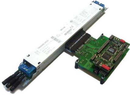
Fig. 14 Photograph of the 35W ballast and the external DSP control board.
