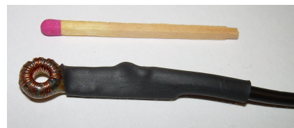
Fig. 9: Self-made AC-current transformer with a sensitivity of 100 mV/A to measure the Drain-Source current I_{DS} of the MOSFET.
