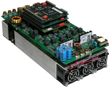
Fig. 2. Photograph of the analyzed RB-IGBT indirect matrix converter (Dimensions: 76 mm x 120 mm x 260 mm).
