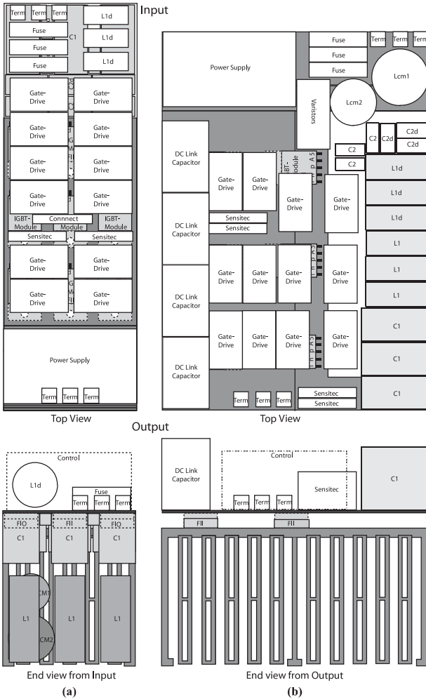
Fig. 9. System layout and construction of (a) VSMC (24.4 cm × 8.0 cm × 11.8cm & volume is 2.3 liters) (b) BBC (22.7 cm × 16.0 cm × 13.4 cm & volume is 4.6 liters)
