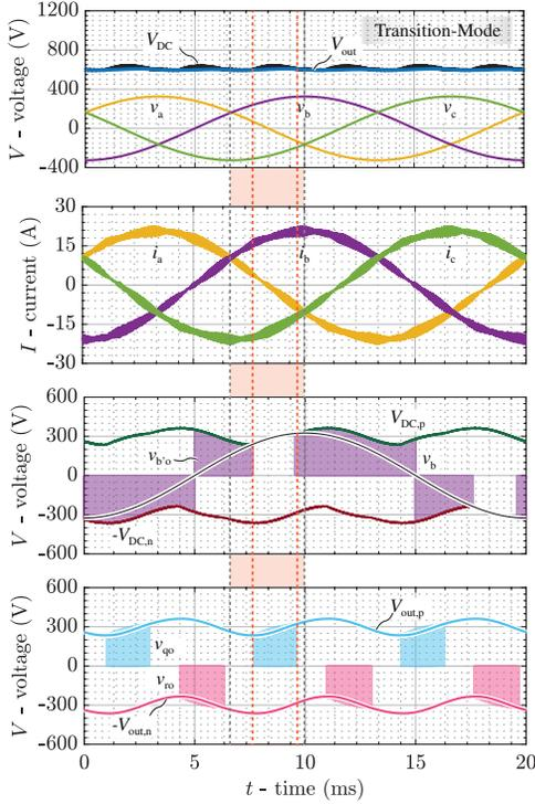
**Fig. 4:** Simulated key waveforms of the non-isolated 3- $\Phi$  Bb voltage DC-link EV charger shown in **Fig. 1** when operating in the transition-mode. One 60°-sector of one mains period ( $v_b > v_a > v_c$ ) is highlighted with a shaded background; note that the converter operates with 1/3-PWM-ZCM in a part of this sector (where the DC/DC-stage's upper HB is HF-switching, delineated by the dashed orange lines) and with 3/3-PWM-ZCM otherwise.
