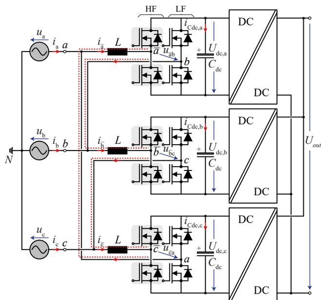
**Fig. 13.** Phase-modular three-phase isolated PFC ac-dc converter system with a delta ( $\Delta$ ) arrangement of the PFC rectifier front-ends [17] (with a typical average dc-link voltage level of  $\bar{U}_{dc} = 700$  V for a grid with 230 V<sub>rms</sub> line-to-neutral voltage): The LF CM current circulating inside the  $\Delta$ -connection (the current path is highlighted with a red dashed line) does not impact the grid currents and allows to alter the LF input power flows of the modules.
