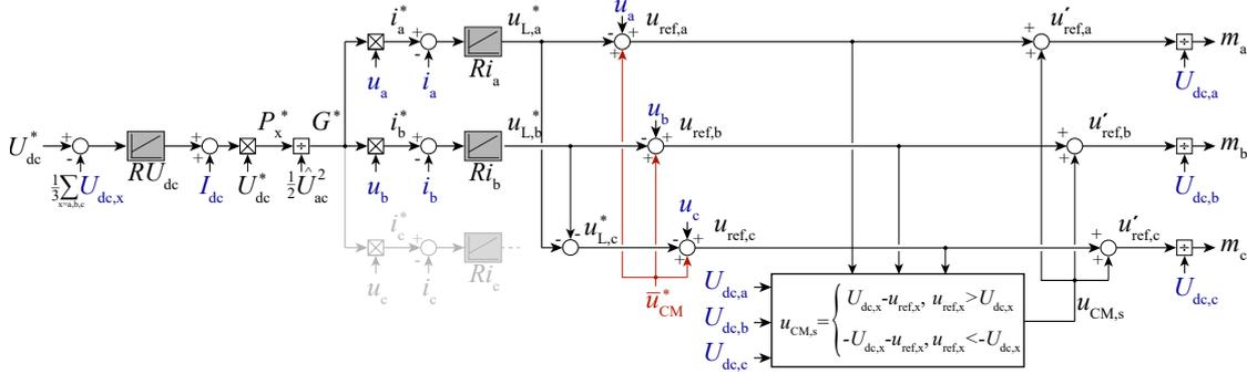
**Fig. 7.** Considered PFC rectifier control structure comprising the saturable CM voltage modulator from [20,25] setting  $u_{CM,s}$  such that in each module  $x$  the LF switch node voltage  $\bar{u}_{\bar{x}\bar{N}}(t)$  remains below the limit imposed by the dc-link voltage  $U_{dc,x}(t)$ , i.e.,  $\bar{u}_{\bar{x}\bar{N}}(t) \in [-U_{dc,x}(t), U_{dc,x}(t)]$ .
