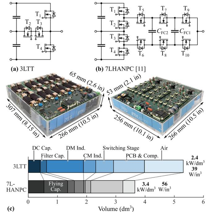
**Fig. 3** 12.5 kW three-phase inverter demonstrator systems realized as (a) all-SiC 3LTT inverter with DC-side CM filter (this work) and, for comparison, (b) as all-Si seven-level hybrid active-neutral-point-clamped/flying-capacitor converter (7LHANPC) [11]. (c) Volume breakdown of the two demonstrator systems. The 3LTT demonstrator's power density is 2.4 kW/dm<sup>3</sup> (39 W/in<sup>3</sup>) and the 7LHANPC prototype's is 3.4 kW/dm<sup>3</sup> (56 W/in<sup>3</sup>).
