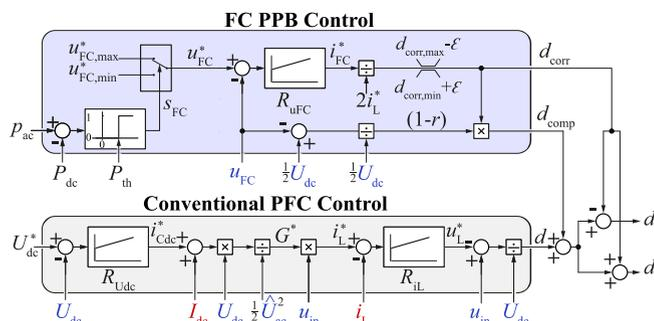
**FIGURE 3.** Considered 3L FC PFC rectifier control concept enabling active FC PPB operation.
