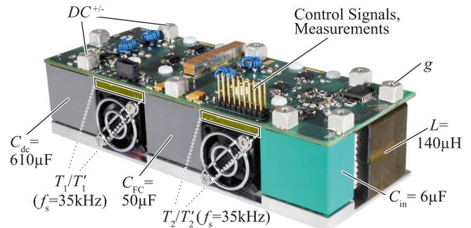
**FIGURE 6.** Employed 3L FC converter prototype (details on the system design can be found in [17] and component designators refer to Fig. 1). The system is connected to an external full-bridge diode rectifier (not shown).
