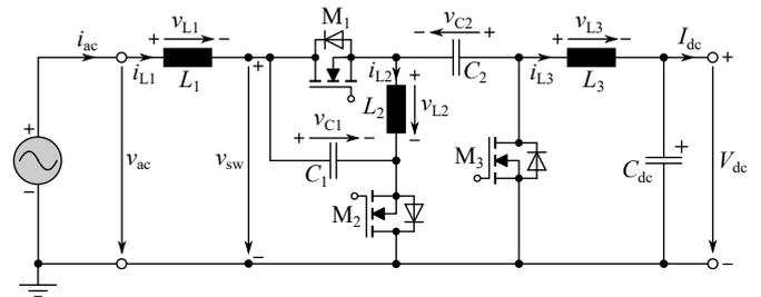
Fig. 1. Main power circuit of the novel bidirectional three-switch single-stage single-phase ac-dc buck-boost converter from [2], providing dc output voltages  $V_{dc}$  above and below grid input voltage amplitude  $\hat{V}_{ac}$ . The considered system specifications are listed in Tab. I.
