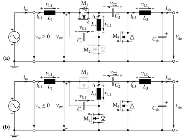
**Fig. 5.** Explanation of the proposed advanced modulation: the proposed three-switch single-stage ac-dc buck-boost converter from **Fig. 1** can operate in two distinct configurations, i.e., in (a) SEPIC mode for  $v_{ac} > 0$  V (the switch  $M_2$  is permanently on), and (b) Ćuk mode for  $v_{ac} \leq 0$  V (the switch  $M_1$  is permanently on). In both cases, only the two respective other transistors are operating with PWM instead of all three transistors as in the conventional modulation.
