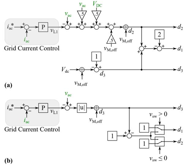
**Fig. 6.** Control diagram for controlling the grid current  $i_{ac}$  for (a) the standard modulation and (b) the advanced modulation. Note that all variables refer to local average values; the  $\langle \rangle$  symbols have been omitted for better visibility.
