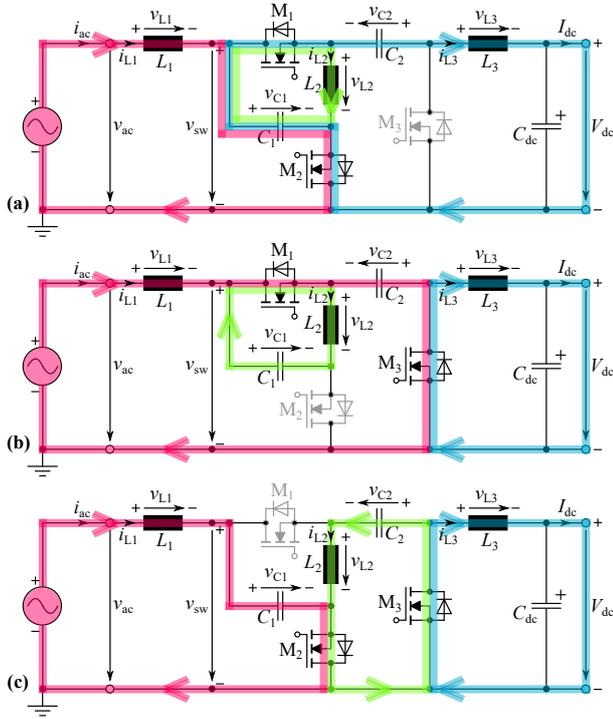
**Fig. 4.** Conduction states of the ac-dc converter from **Fig. 1**. (a)  $s_1 = 1, s_2 = 1$ , (b)  $s_1 = 1, s_3 = 1$ , (c)  $s_2 = 1, s_3 = 1$ , where  $s_{1...3}$  are the gate signals of the corresponding power transistors  $M_{1...3}$ . The colored current paths are for the positive cycle of the grid voltage  $v_{ac}$ .
