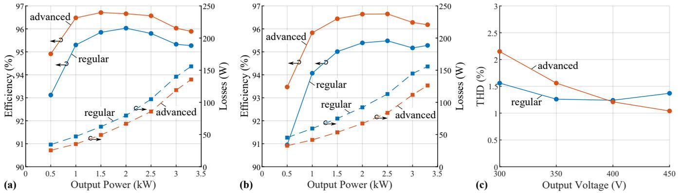
**Fig. 10.** Measured converter efficiencies (round scatter symbols) and power losses (square scatter symbols) over the output power for (a)  $V_{dc} = 300$  V and (b)  $V_{dc} = 450$  V, considering the conventional and the proposed advanced modulation techniques. (c) Total Harmonic Distortion ( $THD_{40}$ ) for different output voltage levels and nominal power ( $P_{out} = 3.3$  kW).
