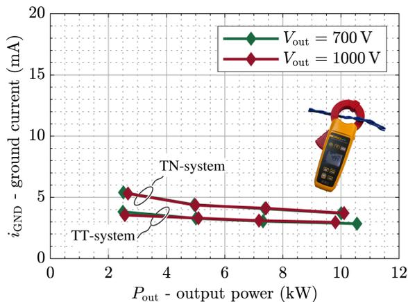
**Fig. 15:** Ground current  $i_{GND}$  measured with a leakage current clamp meter *Fluke 368 FC* [39] for operation with two different output voltages and various power levels from 25% to 100% of rated load. For both grounding schemes (TT and TN), the measured ground current remains far below RCD trip levels of 30 mA.
