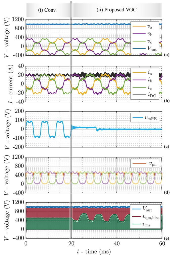
**Fig. 19:** Simulated key waveforms for operation in the boost-mode with distorted mains voltages (i.e., the 3- $\Phi$  mains voltages contain 12% of 5th, 10% of 7th, and 7% of 11th harmonics [44]), (i) regulated by conventional synergetic control without VGC and (ii) with the proposed VGC, where  $V_{out} = 1000$  V and  $P_{out} = 10$  kW.
