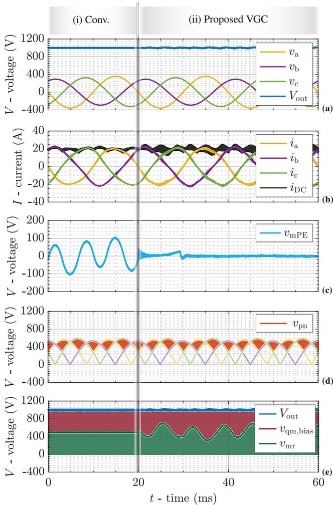
**Fig. 18:** Simulated key waveforms for operation in the boost-mode under asymmetric 3- $\Phi$  mains voltage amplitudes, e.g., +10% in phase  $a$  and -10% in phase  $b$ , (i) regulated by conventional synergetic control without VGC and (ii) with the proposed VGC, where  $V_{out} = 1000$  V and  $P_{out} = 10$  kW.
