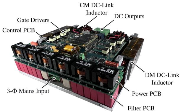
**Fig. 10:** Photo of the realized 10 kW 3- $\Phi$  current DC-link buck-boost PFC rectifier (see Fig. 3) hardware demonstrator, which interfaces a 400 V mains and a DC output voltage in the range of 300 V to 1000 V; detailed specifications are given in Tab. I. Employing 1200 V SiC (CSR-stage) and 900 V SiC (DC/DC-stage) MOSFETs, the converter achieves a power density of 6.4 kW/dm<sup>3</sup> (184×172×49 mm<sup>3</sup>) or 107.5 W/in<sup>3</sup> (7.2×6.8×1.9 in<sup>3</sup>).
