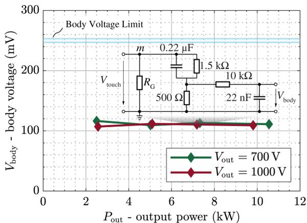
**Fig. 16:** Body voltage  $V_{\text{body}}$  obtained by processing the measured touch voltage  $V_{\text{touch}}$  with the transfer function of the human body impedance network according to UL 2202. The converter operates with the proposed GCC at  $V_{\text{out}} = 700 \text{ V}$  and  $V_{\text{out}} = 1000 \text{ V}$ , considering different output power levels. In all cases, the measured body voltages of around 110 mV are well below the safe level of 250 mV defined in UL 2202 [2].
