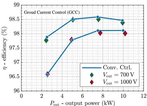
**Fig. 17:** Measured (Yokogawa WT3000) efficiencies of the 10 kW hardware demonstrator (see Fig. 10) with  $V_{\text{out}} = 700 \text{ V}$  and  $V_{\text{out}} = 1000 \text{ V}$  (i.e., boost-mode) and for various output power levels. Enabling GCC has almost no impact on the efficiency; and with or without GCC a high peak efficiency of about 98.5% is achieved.
