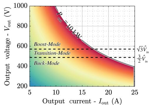
**Fig. 2:** Typical operating range of EV chargers, including a constant output current  $I_{out} = 25$  A region when  $V_{out} < 400$  V and a constant output power  $P_{out} = 10$  kW when  $V_{out} > 400$  V. Three operating modes, i.e., buck-mode, boost-mode and transition-mode, are required to cover such a wide output voltage range [20].
