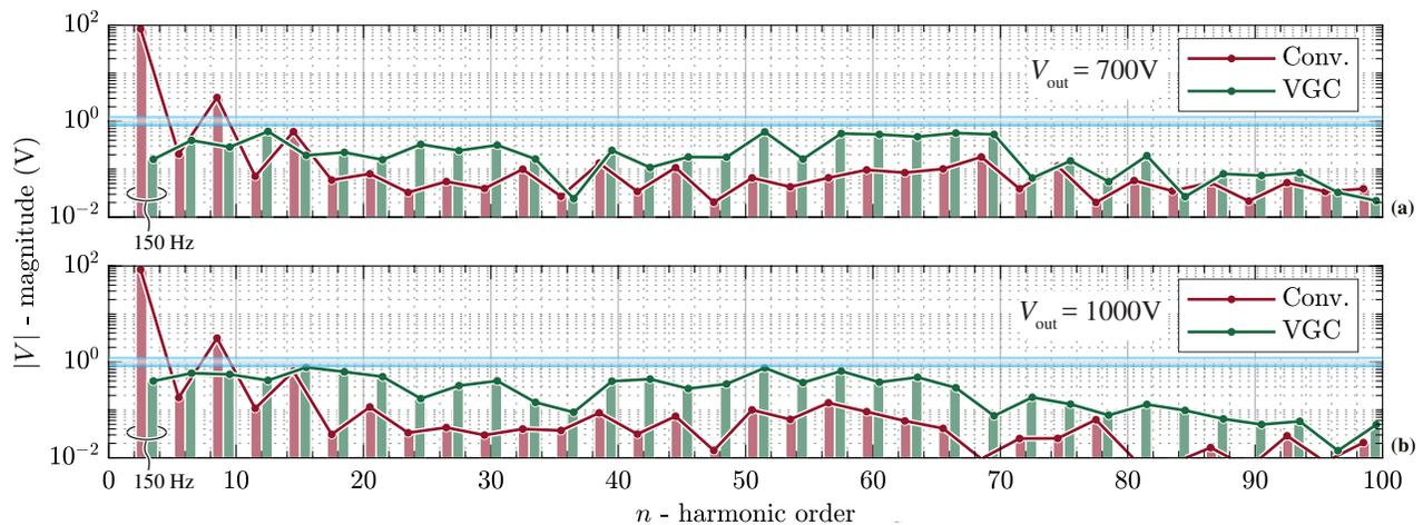
**Fig. 13:** Comparison of the harmonic spectra calculated from measured  $v_{mk}$  when operating without (**Fig. 11**) and with (**Fig. 12**) the proposed VGC at (a)  $V_{out} = 700\text{ V}$ ,  $P_{out} = 4.5\text{ kW}$  and (b)  $V_{out} = 1000\text{ V}$ ,  $P_{out} = 9.1\text{ kW}$ ; in all cases from a 50 Hz mains. Note that VGC successfully suppresses LF CM voltage harmonics, i.e., especially the third-harmonic component is reduced from 80 V without VGC to less than 1 V with VGC.
