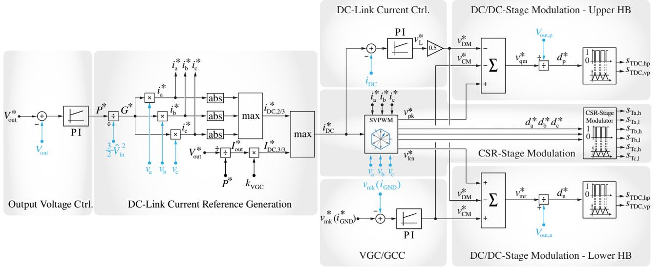
**Fig. 9:** Proposed control block diagram for the 3- $\Phi$  bB current DC-link PFC rectifier system shown in **Fig. 3**. It is based on the synergetic control concept from [20] but in addition implements virtual grounding control (VGC) or ground current control (GCC). The functionality and the interaction of the individual control blocks are described in the text. Note that all quantities refer to local average values here.
