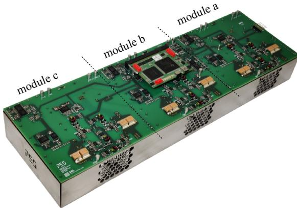
**Fig. 5.** Phase-modular three-phase PFC rectifier hardware prototype which can be configured for Y- and Δ-connected operation of the modules as highlighted in Fig. 3. The system dimensions are 395 mm × 125 mm × 50 mm (15.6 in × 4.9 in × 2.0 in) and details on the main power components are listed in Tab. 2.
