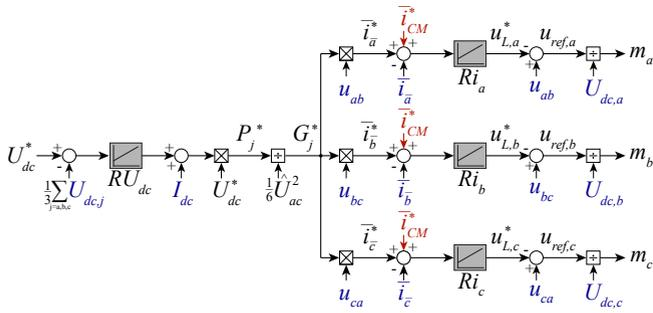
**Fig. 8.** Block diagram of a cascaded control of the PFC rectifier input stages of **Fig. 3(e)** considering a 3<sup>rd</sup> harmonic CM current injection  $\bar{i}_{CM}^*$ .
