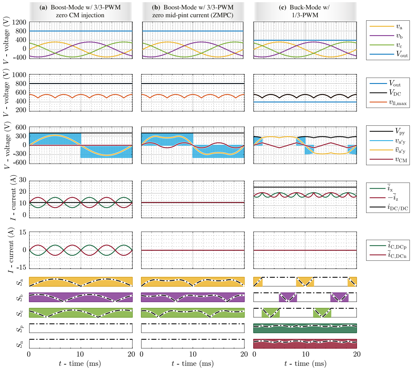
Fig. 3: Exemplary key waveforms for operating over a wide output voltage range, i.e., buck-boost operation, of the considered 3- \Phi Bb voltage DC-link PFC rectifier system shown in Fig. 2 . In the boost-mode, the VSR-stage operates with 3/3-PWM to ensure 3- \Phi sinusoidal mains currents and regulate the output voltage. (a) 3/3-PWM can be implemented with zero LF CM injection, however, LF capacitive currents (up to 4 A) flow through the DC-link capacitors (note that the DC-link capacitors are replaced with ideal voltage sources such that these LF DC-link capacitor currents do not result in LF DC-link voltage variations). Thus, (b) another variety of 3/3-PWM with LF CM voltage injection that ensures zero mid-point current (ZMPC) [19] and hence zero LF DC-link capacitor currents is implemented. (c) In the buck-mode, the VSR-stage operates with 1/3-PWM [8], where the DC/DC-stage controls the DC-link voltage to follow the six-pulse shape of the upper envelope of the line-to-line voltage absolute values and hence only one of the VSR-stage's three HBs operates with HF PWM at any given time.
