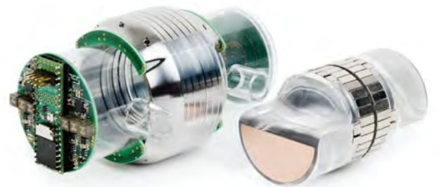
Fig. 15: Complete hardware prototype of the ShuttlePump with its drive system, consisting of the drive and control unit, linear-rotary position sensors [8] and the LiRA (stator and mover).
