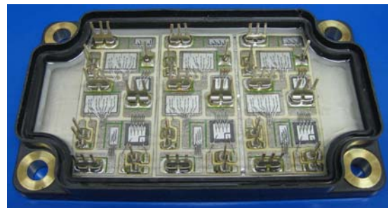
Fig. 5 Picture of the open Microsemi power module
