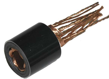
Figure 1. Generator with rotor removed. The cup-shaped litz-wire winding and low loss stator core can be seen.
